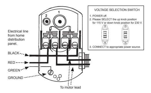
We recommend that a licensed electrician be employed to do the proper wiring to the pressure switch, and to permanently ground the motor in accordance to the electrical codes in your area.
